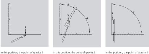
is furthest away from the pivot point. The strongest force is required for opening the flap. Both strokes are compressed. The cylinder with the stronger force opens it.
