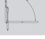
In this position, the point of gravity S is close to or directly on the pivot point. A weak spring force is required. Both strokes are fully extended.
