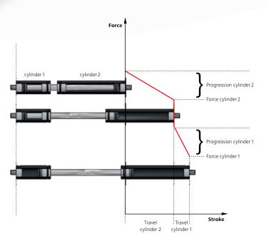
Hahn Gasfedern has developed special double-stroke springs for heavy flaps with a large opening angle, which are characterized by a low starting and a high ultimate force. These springs have two pressure cylinders that can be filled differently and thus are able to cover two force ranges. The compression of the piston rod generates a bent characteristic curve, which can be better adjusted to the force progression of the flap.
